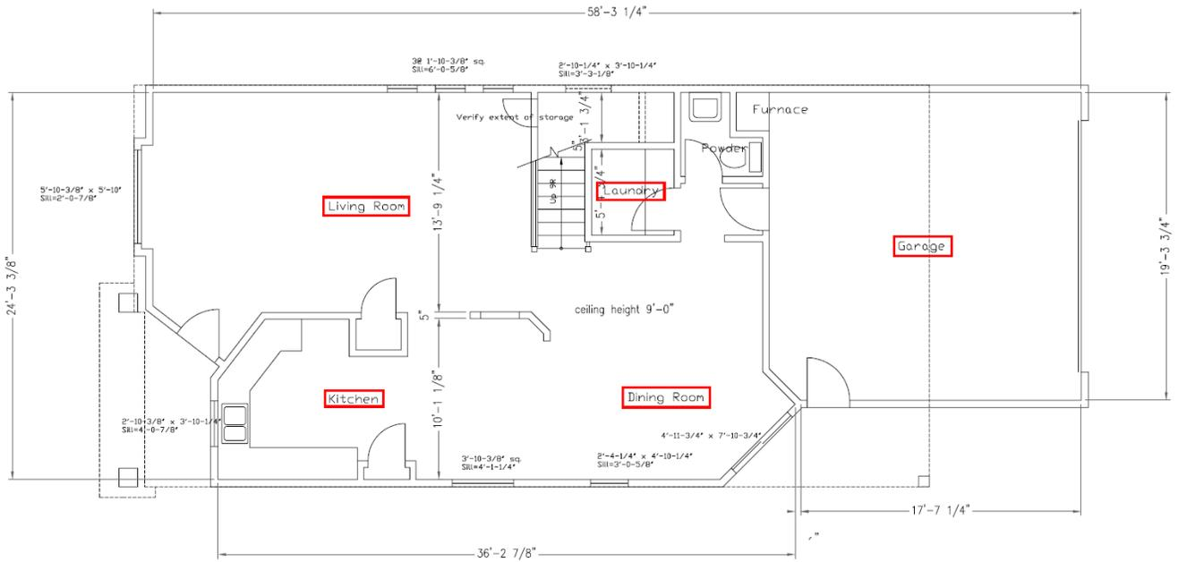
FIGURE 16. CALEB FLOOR PLAN – LOWER FLOOR
