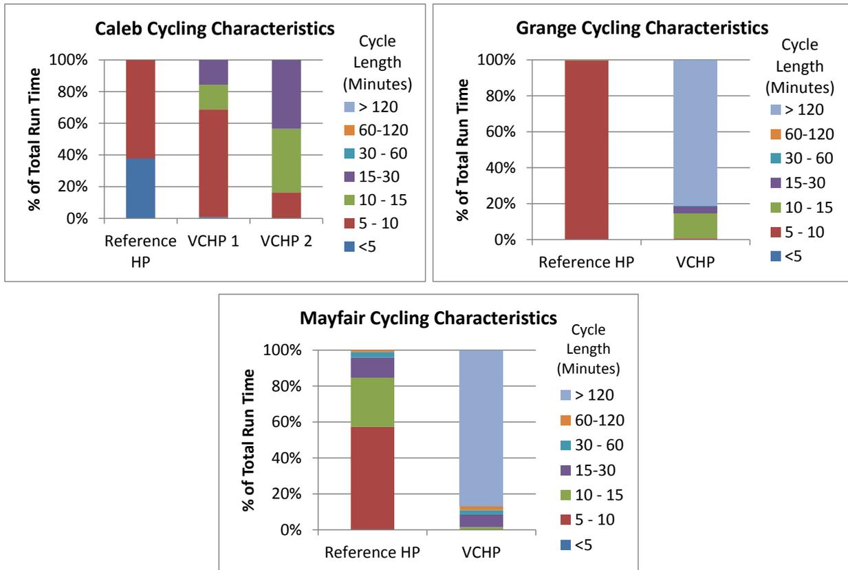
FIGURE 29. COOLING MODE CYCLING CHARACTERISTICS (CONSTANT SETPOINT DAYS??)
