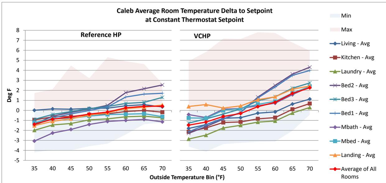
FIGURE 39. CALEB ROOM TEMPERATURES DURING CONSTANT SETPOINT HEATING
