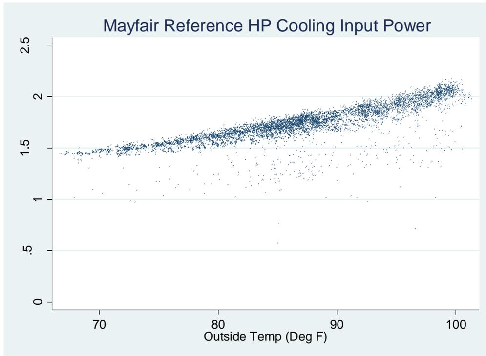
FIGURE 53. MAYFAIR REFERENCE HEAT PUMP IN COOLING MODE
