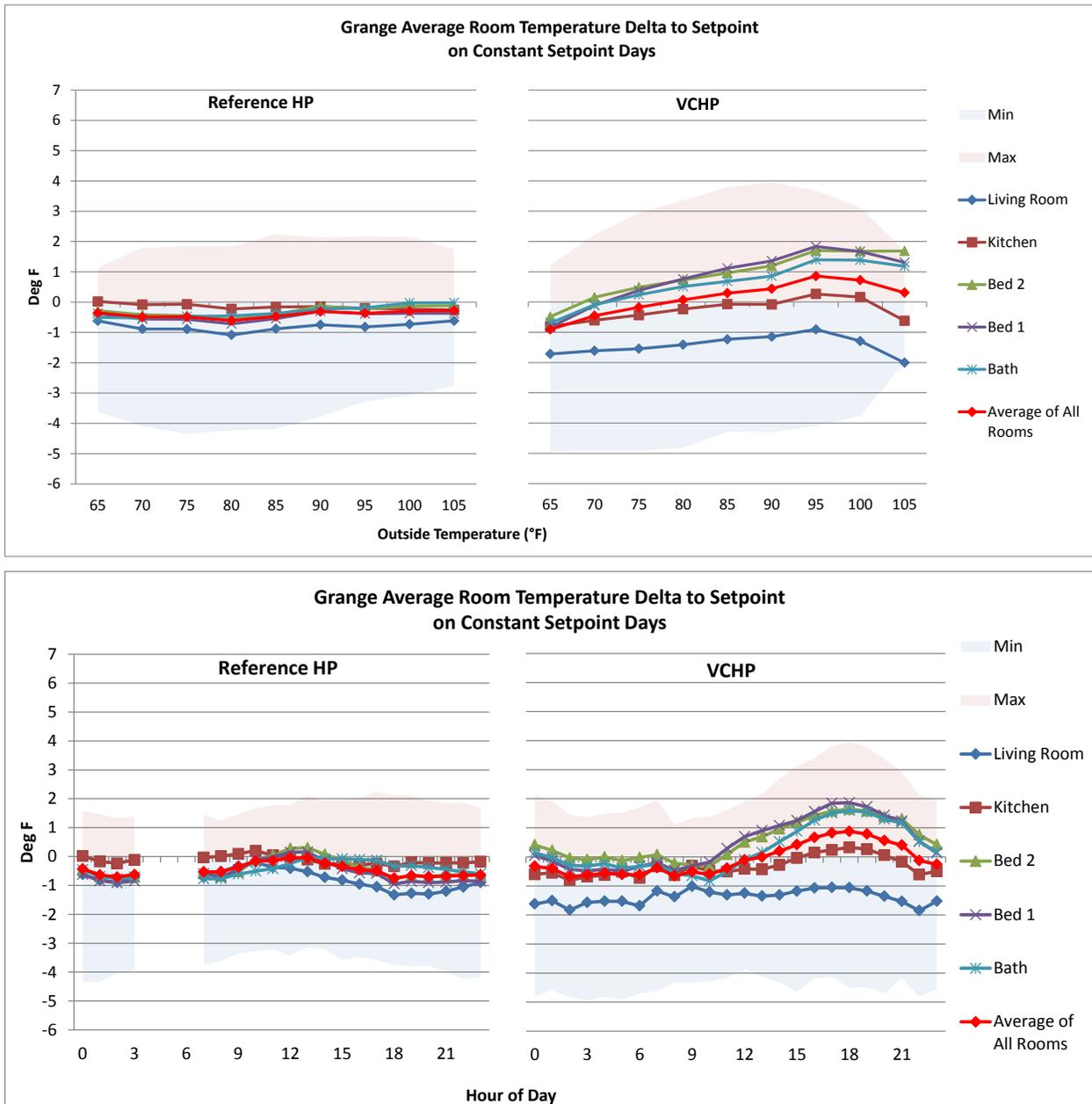
FIGURE 25. GRANGE ROOM TEMPERATURES DURING CONSTANT SETPOINT COOLING
