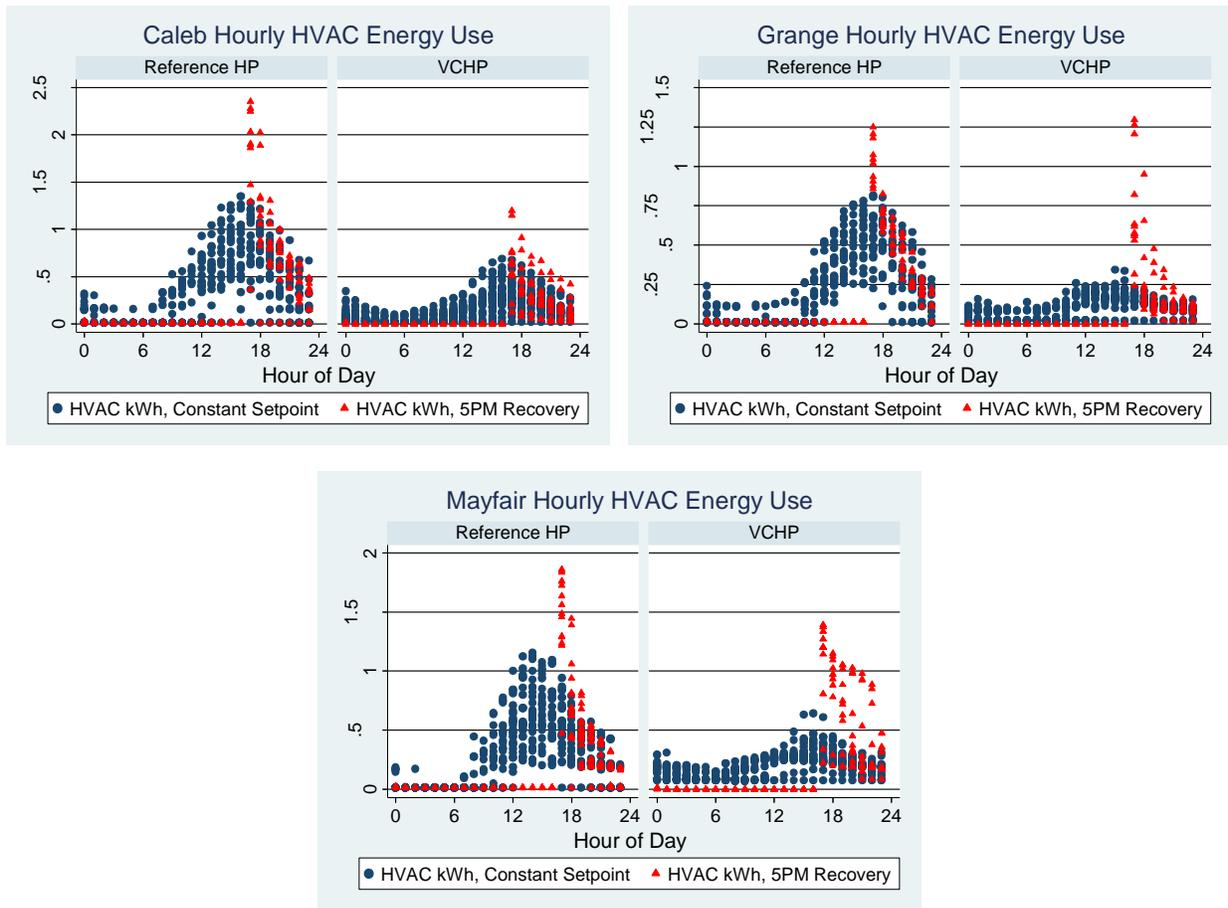
FIGURE 36. HOURLY COOLING ENERGY USE PROFILES
