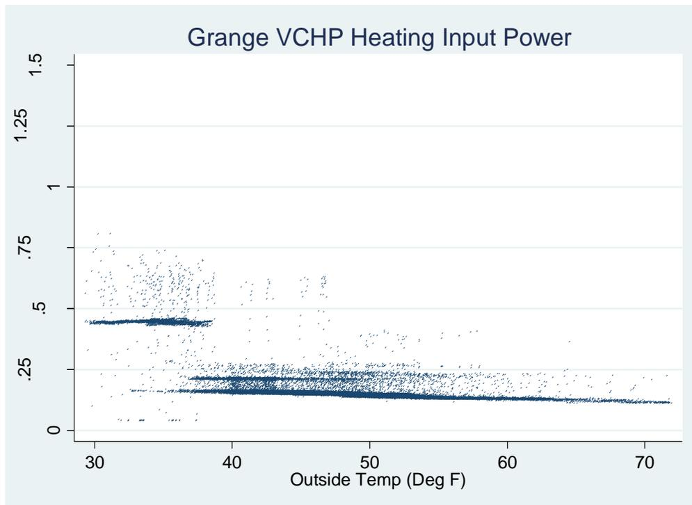
FIGURE 52. GRANGE VCHP IN HEATING MODE
