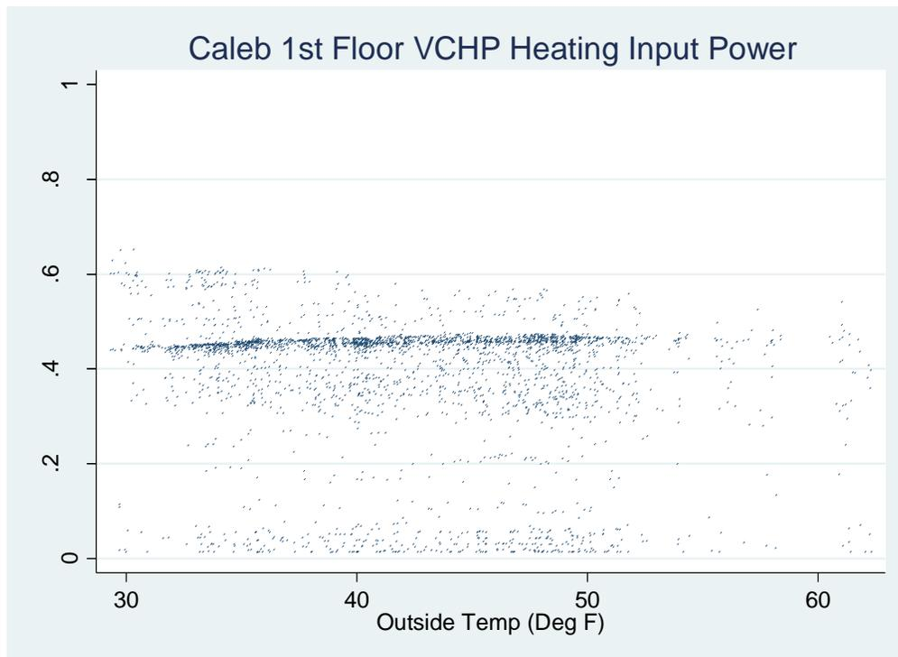
FIGURE 46. CALEB 1<sup>ST</sup> FLOOR VCHP IN HEATING MODE
