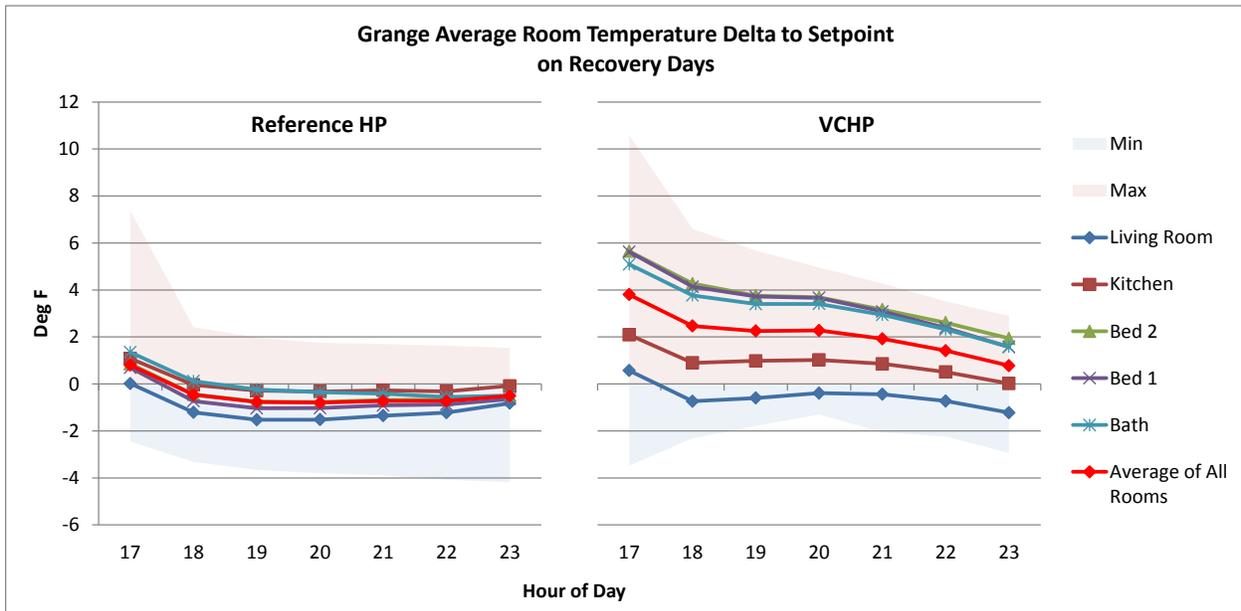
FIGURE 31. GRANGE ROOM TEMPERATURES DURING COOLING RECOVERY
