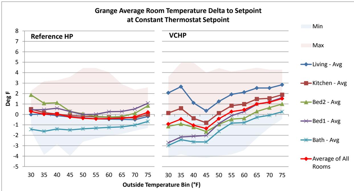
FIGURE 40. GRANGE ROOM TEMPERATURES DURING CONSTANT SETPOINT HEATING
