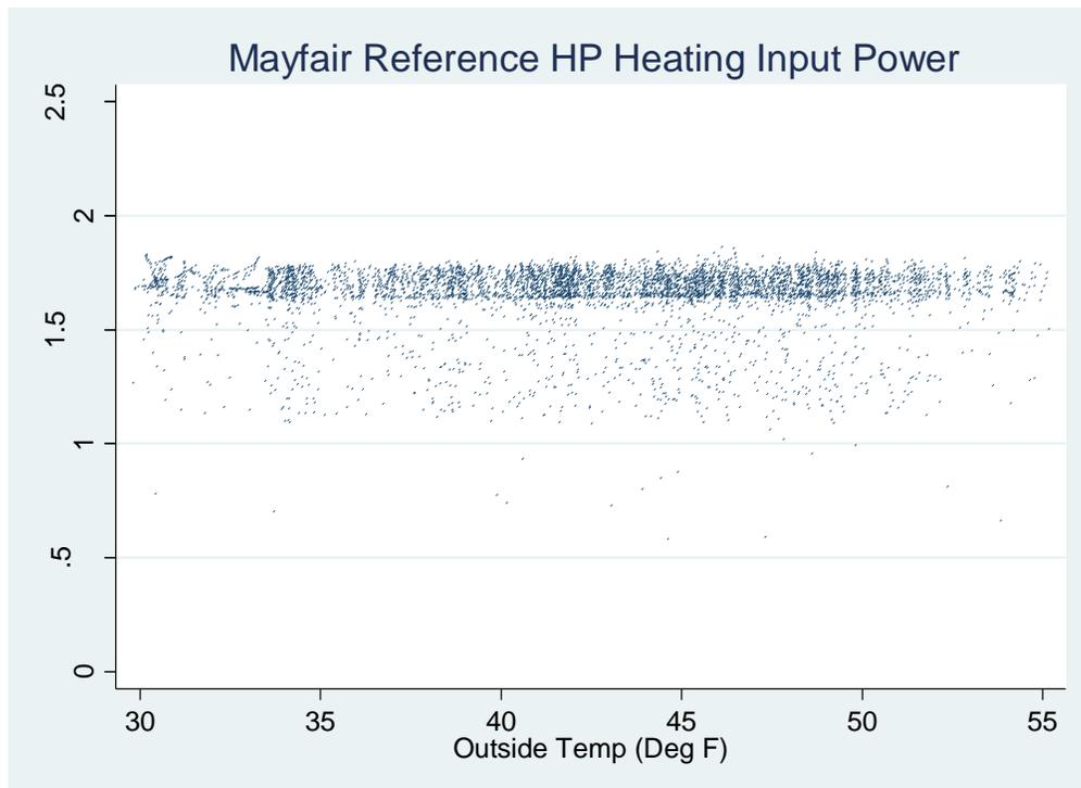
FIGURE 54. MAYFAIR REFERENCE HEAT PUMP IN HEATING MODE
