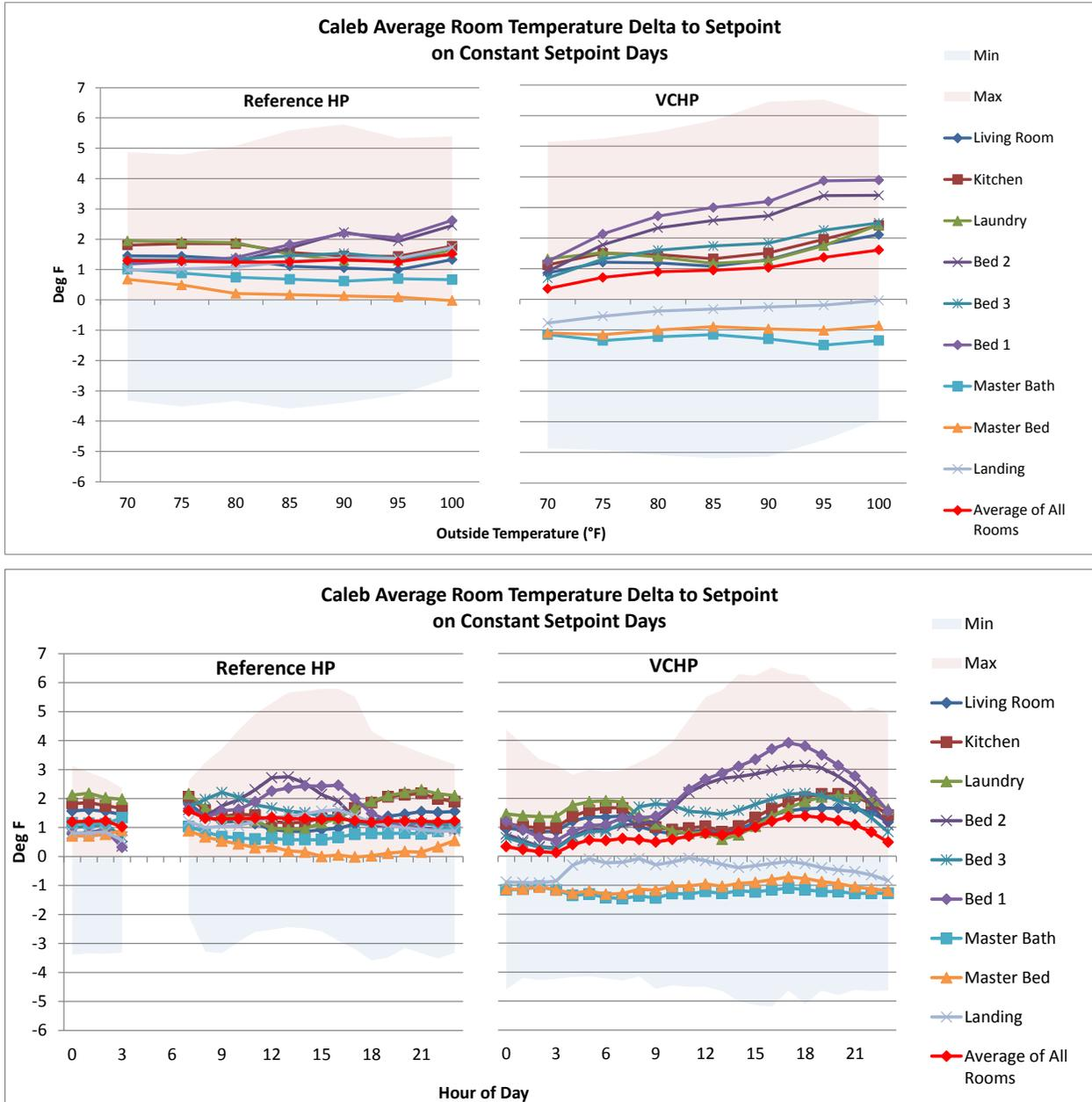
FIGURE 24. CALEB ROOM TEMPERATURES DURING CONSTANT SETPOINT COOLING
