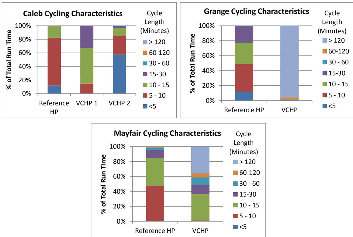
FIGURE 42. HEATING MODE CYCLING CHARACTERISTICS
