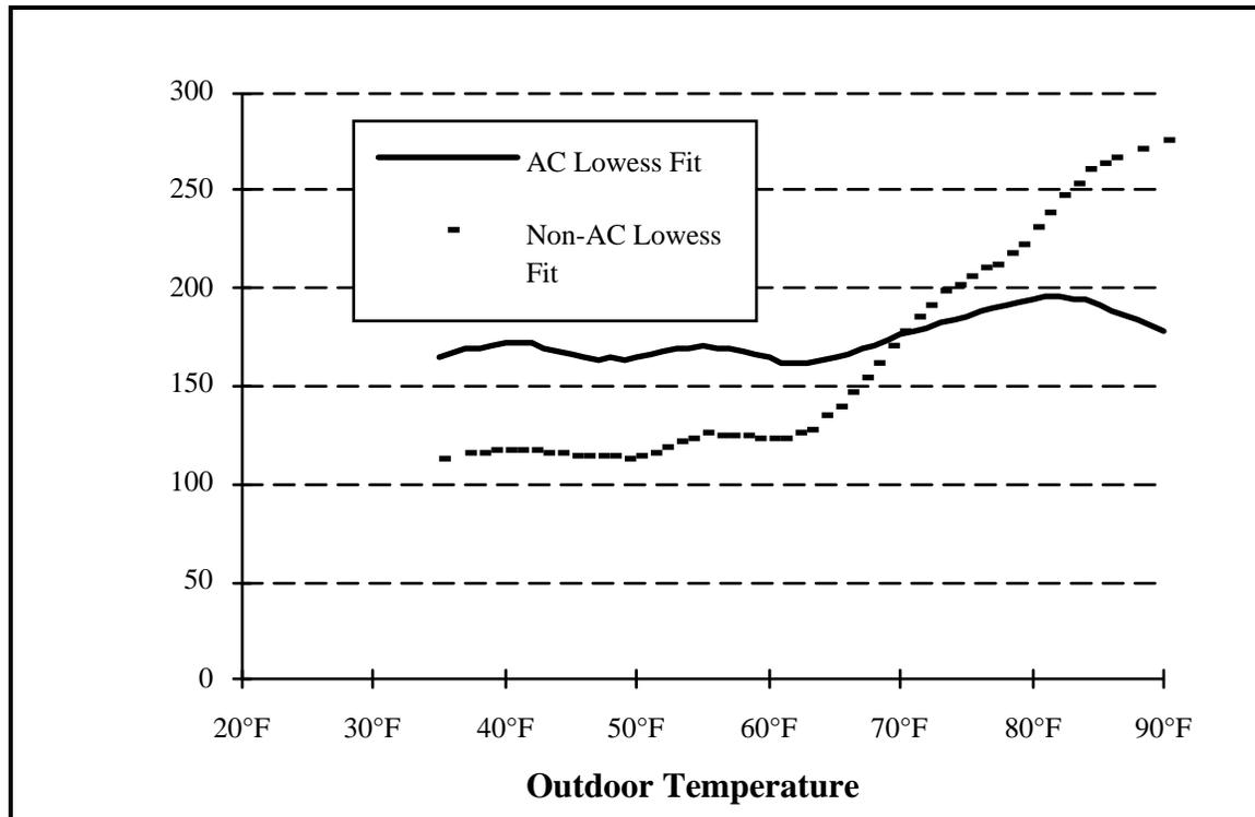
**Figure 7. Standard Deviation of Consumption vs. Outdoor Temperature**
