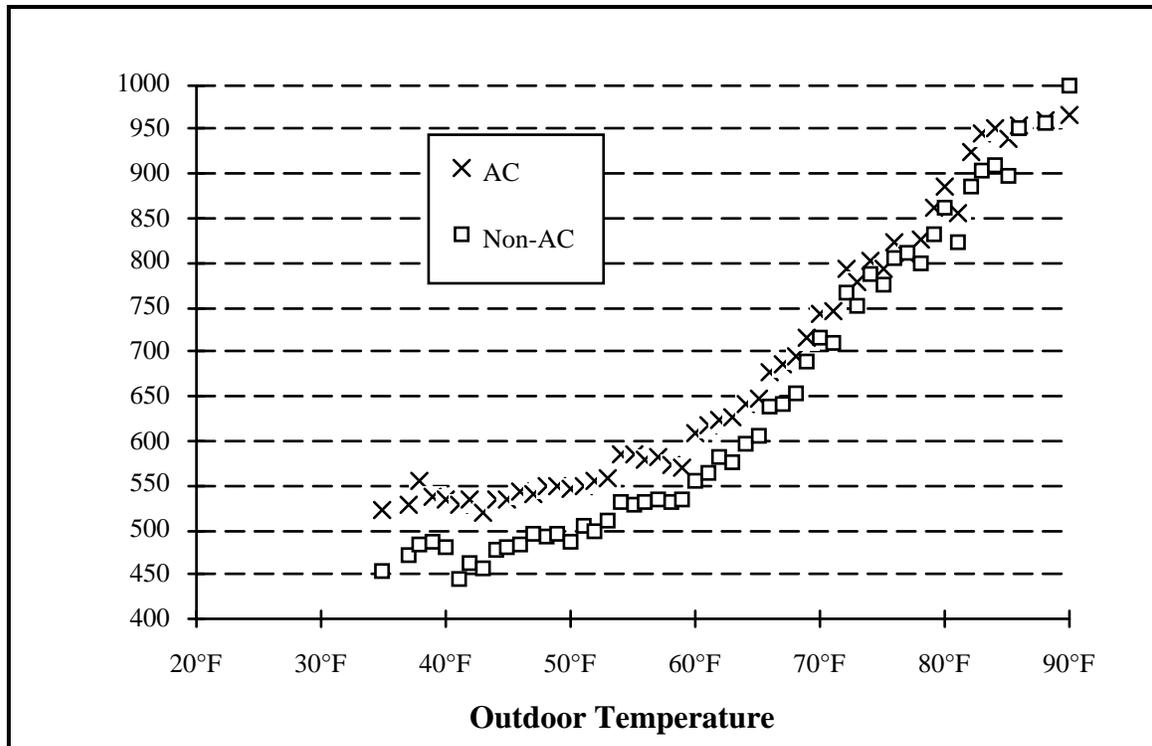
**Figure 5. Effect of AC and Temperature on Refrigerator Energy Consumption**
