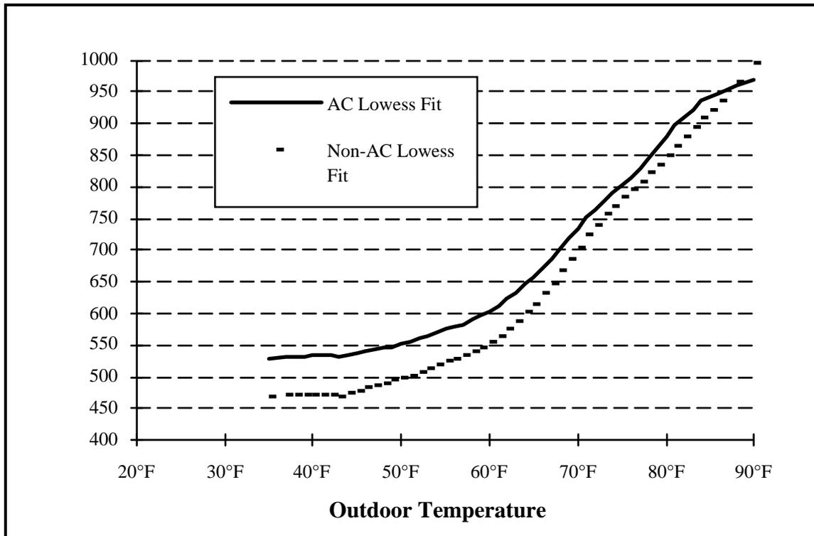
**Figure 6. Smoothed Data - AC and Temperature vs. Consumption**
