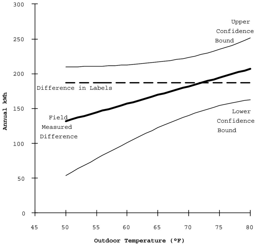
The confidence interval is smallest at the mean of the sampled data. As the sample grows to include data in cooler weather, the precision of the estimate will be improved and the confidence band narrowed.
