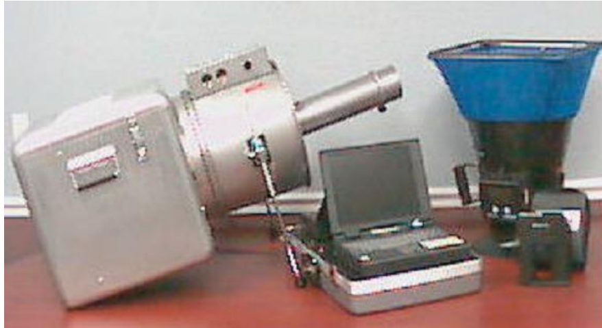
Figure 2.1.1: Aerosol sealing machine, computer-control suitcase, and diagnostic tools (flow capture hood, and infrared laser-guided temperature-measurement gun)
