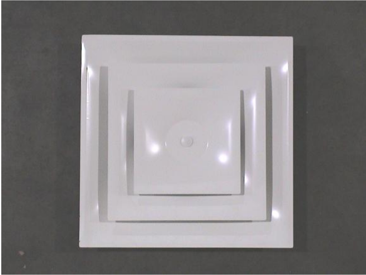
Figure B.8: Fin diffuser, many of which can be sealed temporarily by removing fins and plugging opening with foam. (courtesy of Lawrence Berkeley National Laboratory)
