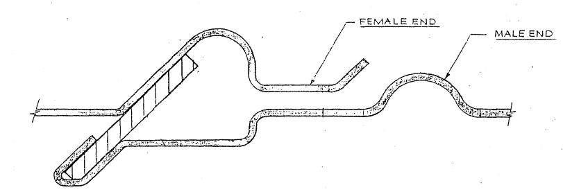
PEG constructed two connection prototypes, a rigid sheet metal duct and a helix core flex duct, and conducted laboratory tests to determine each one's leakage. The first design tested was a 6 inch diameter round sheet metal duct constructed with 26 gauge material. This is the same material used in current residential systems. The second was a helix core flex duct fitting over a 6 inch diameter sleeve.
