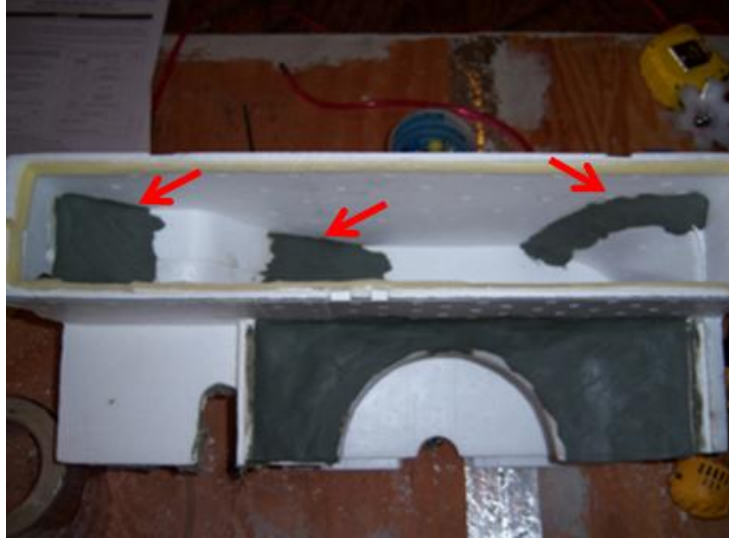
Figure 50 Indoor Fan Housing with Smoothed Outlet Transitions
