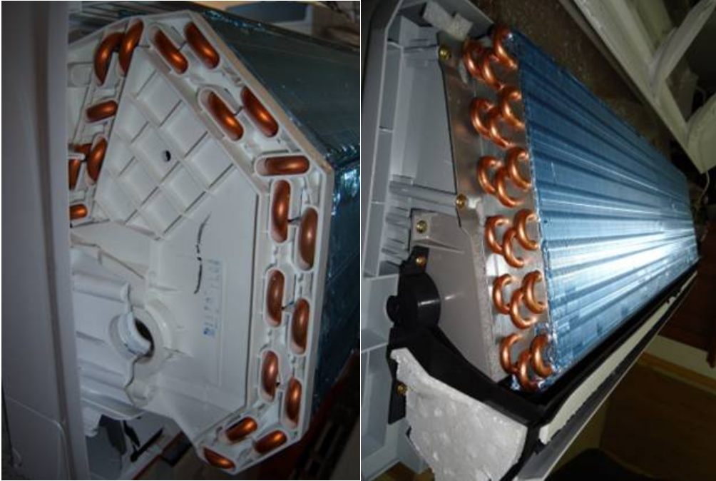
Figure 54 US (left) and Saudi Arabia Baseline (right) Mini Split Evaporator Coils
