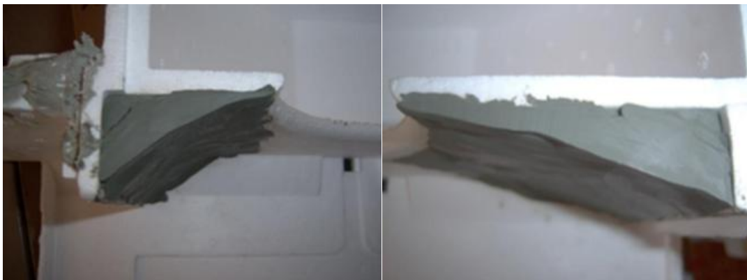
Figure 49 Indoor Fan Inlet with Smoothed Inlet Transitions
