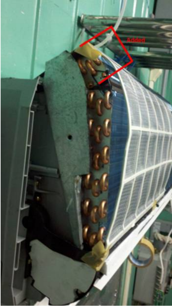
Figure 63 Mini Split AC Prototype Evaporator Coil Enlarged
