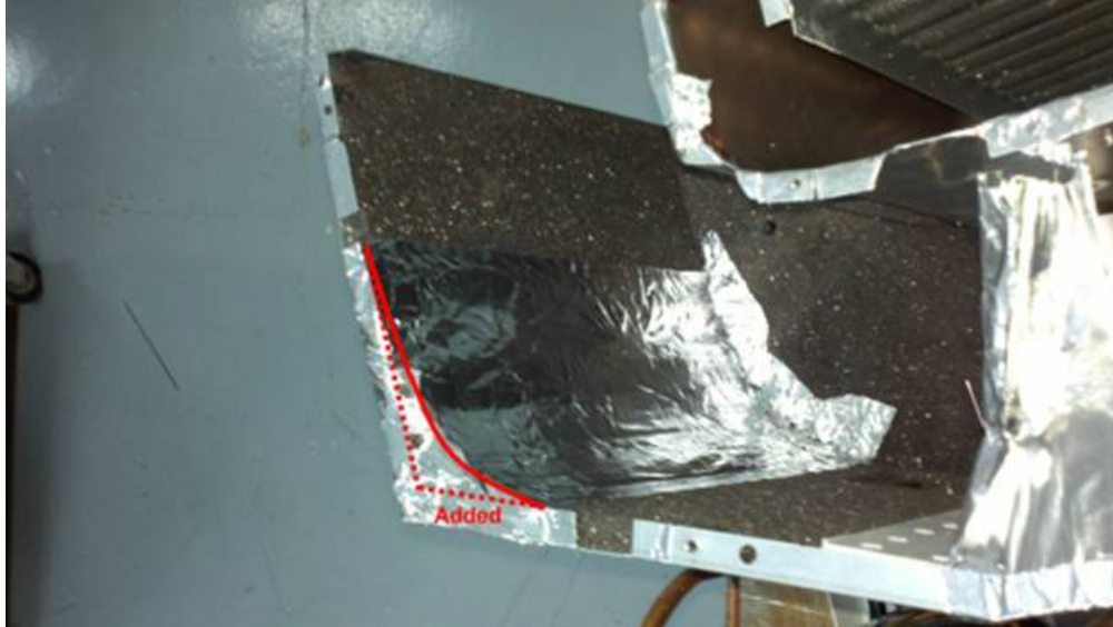
Figure 57 Window AC Prototype Indoor Fan Outlet Smoothing
