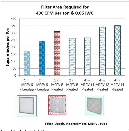
Figure 59: Required Air Filter Area for 400 CEM per Ton at 0.50 IWC
