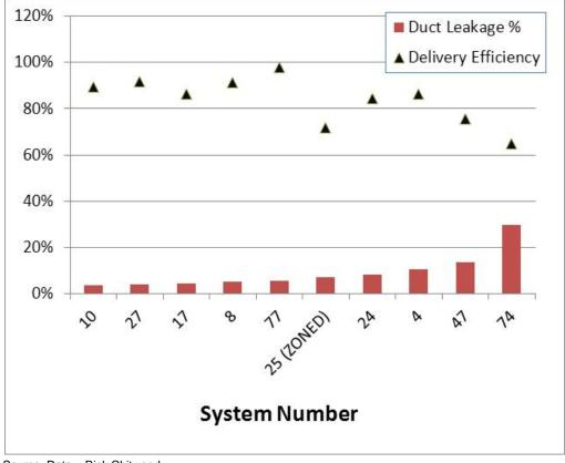
Figure 28: Delivery Efficiency and Duct Leakage
