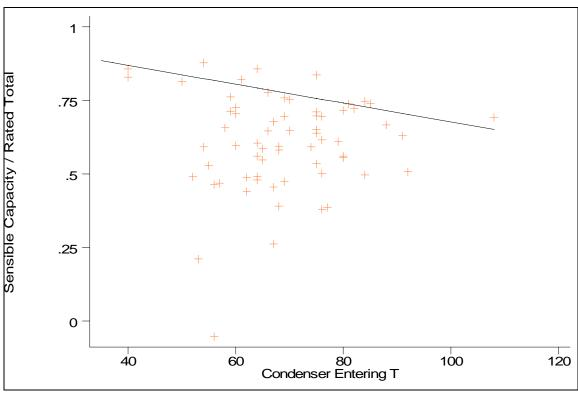
Figure 5: Sensible Capacity vs. Outdoor Temperature
