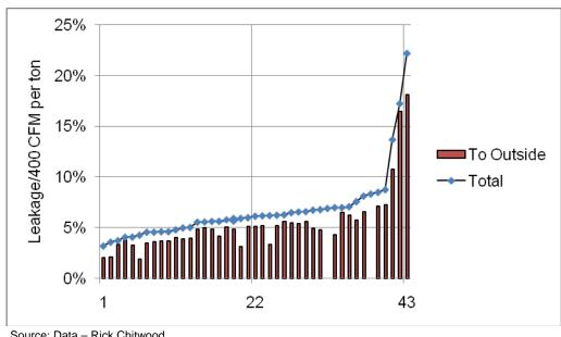
Figure 21: Duct Leakage for Single-Family Buildings
