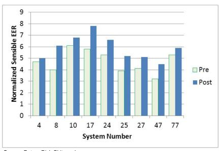
Figure 27: Normalized Sensible EER from Measurements at the Registers
