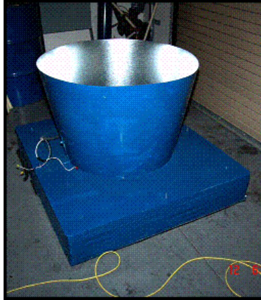
Figure 46. Diffuser for Condenser Fan
