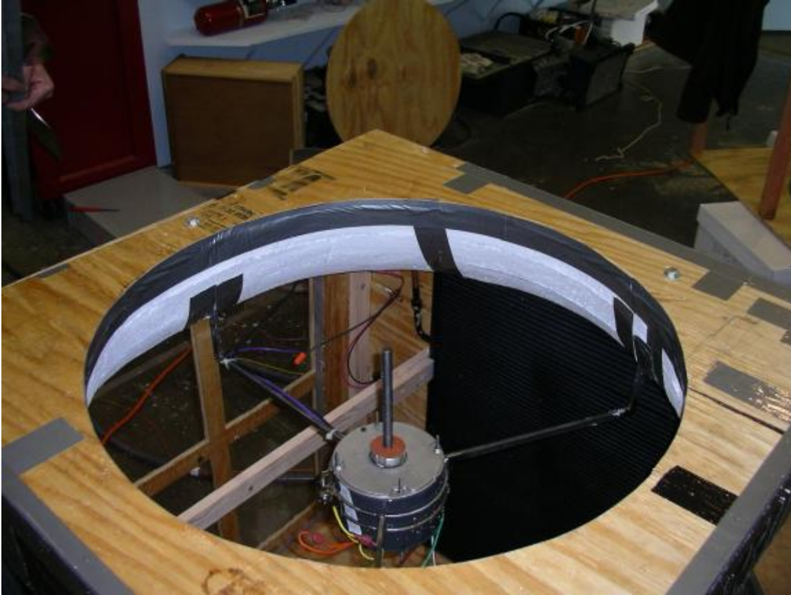
Figure 45. Shaped Inlet for Condenser Fan
